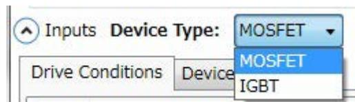
From the Device Type drop-down list, select a device type.
