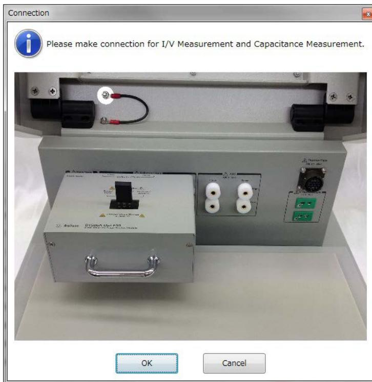
1. Set the 3-pin inline package socket module and other accessories corresponding to the DUT and then set the DUT.
