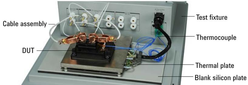
In the above picture, the blank silicon plate is set on the DUT stage, and the Thermal Plate is placed on the plate and connected to the Thermal Plate connector. Also, the thermocouples are connected to the K Thermocouple terminals and put on the places to monitor temperature. For the Thermal Plate, contact inTEST Corporation.
