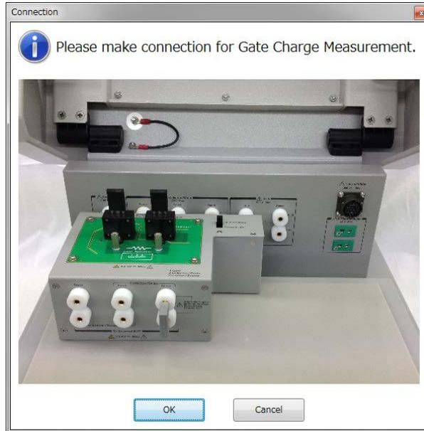
1. Open the test fixture cover, and disconnect the socket module and other accessories from the test fixture.
